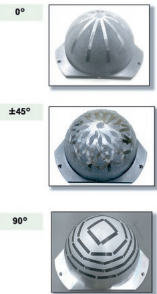
Figure 1 Examples of applying tow prepreg to semi-cylindrical and dome shapes.
