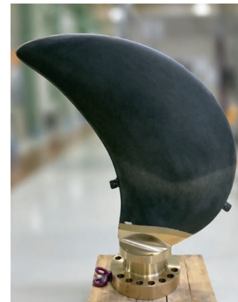
Controllable-pitch propeller featuring a metal core-bonded structure (CFRP blade prototype)
