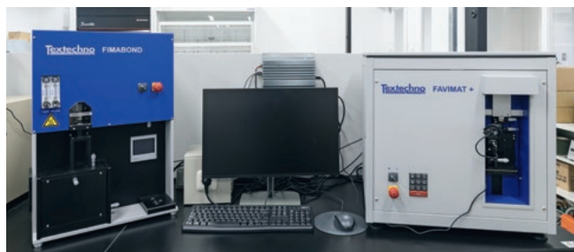
Figure 1 FIMATEST (Left: FIMABOND, right: FAVIMAT+)
