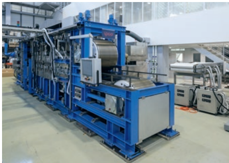
Figure 1 Double belt press system used for continuous preparation of sheet-like intermediate materials
