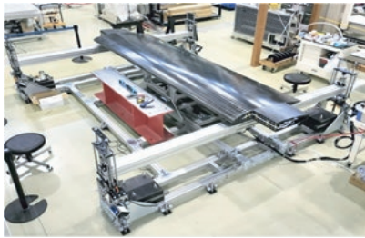
Figure3 Structural load test of the aircraft center wing section.
