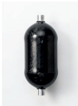
Figure 3 Tank after consolidation by LP-RTM (Molded tank)
