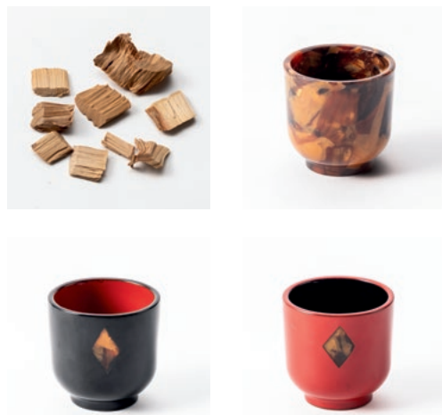
Figure 1 A small cup (top right) made by impregnating waste wood chips (top left) obtained by wood flow forming with thermosetting resin, and prototypes (bottom) which are coated with Yamanaka lacquerware
