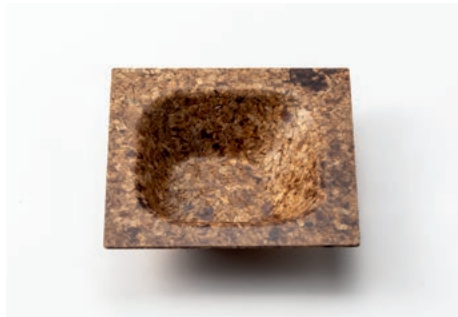
Figure 2 The three-dimensional products obtained by wood flow forming of waste wood in the Yamanaka lacquerware industry; the waste woods are impregnated with thermoplastic resin, which have distinctive designs derived from original woods.
