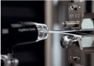
Figure 1 Mode I in double cantilever beam (DCB) setup: fixture for GIC test with video recording option
