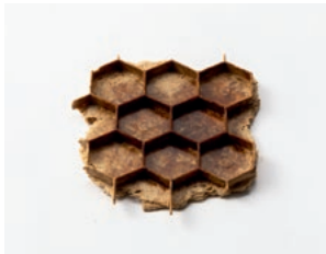
Figure4 Example of the wood flow molding with complex rib geometry
