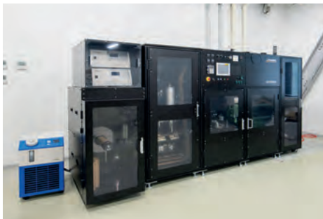
Figure 1. Thermoplastic resin impregnation system for UD Tape using ultrasonic wave
