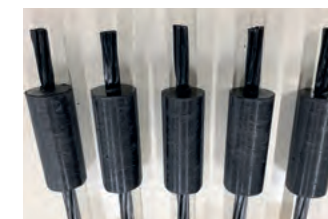
Figure 3. Molded strands with a diameter of 6φ
