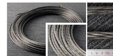
Figure 3. The BFPP with increased diameter by twist
