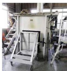
Test of FRP sandwich panels in a refractory furnace
