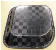
3D shaped sandwich (woven CFPP/PP foam/woven CFPP)
