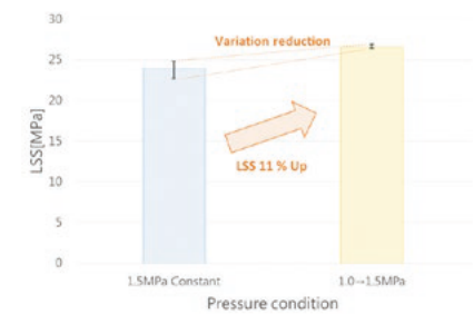
Figure 6. Influence of pressure on welding strength during cooling process
