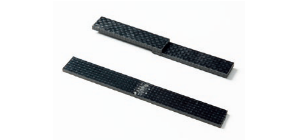
Figure 2. Butt bonding of CFRTP by laser irradiation
