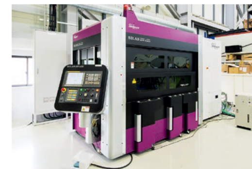
Experimental apparatus: Fiber laser processing machine SPF320 / SFX1800 made by Shibuya Co.
