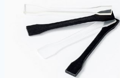
Figure9. PP / PLA alloy test pieces
