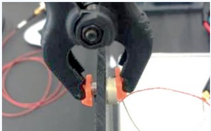
Figure5. Setup for ultrasonic measurements of continuous molding composites
